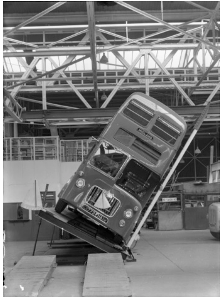
Above: a D9 undergoes a tilt test Left: a mock-up of the D10 design
